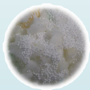
Mixed filling 50% Polystyreen grains 50% Foam flakes
